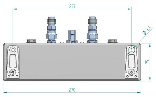
The through holes for all wall brackets are 6.5 mm in size.
