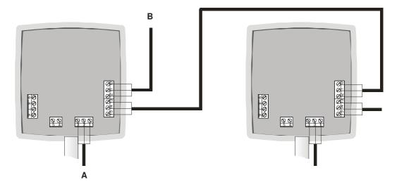
The power supply (24 V DC) is connected up using the "A" cable. Cables must be terminated with wire end ferrules.
