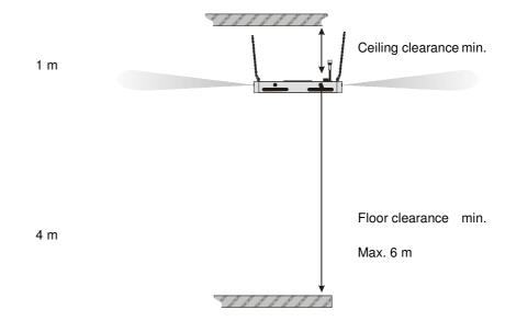
When positioning, ensure that you can keep baffles out of the aerosol mist radius. A corridor between the nozzles – where stanchions are located, for example – is acceptable.
