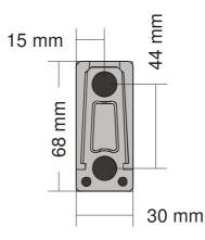
The through holes for all wall brackets are 6.5 mm in size.
