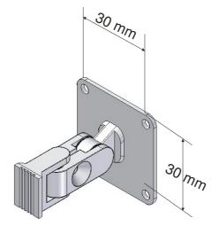
The through holes for all wall brackets are 3.5 mm in size.
