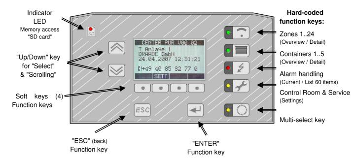
The HumCenter consists of a display and multiple function keys, which can be used to access, select and work with the various menu items. The unit's functionality is described below. For a detailed description of the individual menu items and their parameters, please see the HumDigital operating instructions.
