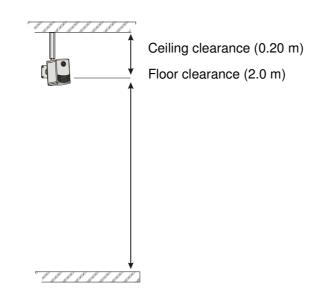
The details given refer to the wall bracket and must be taken as minimum values.
