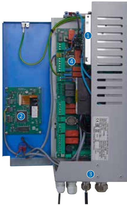
Power supply [1] Control board [2] Powder coated housing [3] Spa Control [4]
