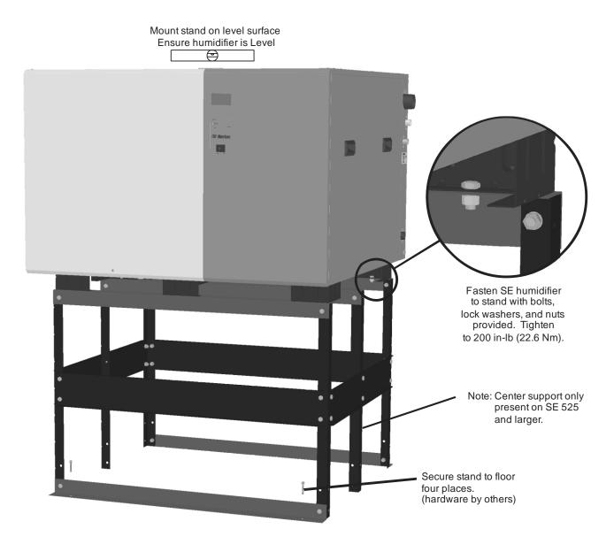
Figure 8: Mounting on Floor Stand
