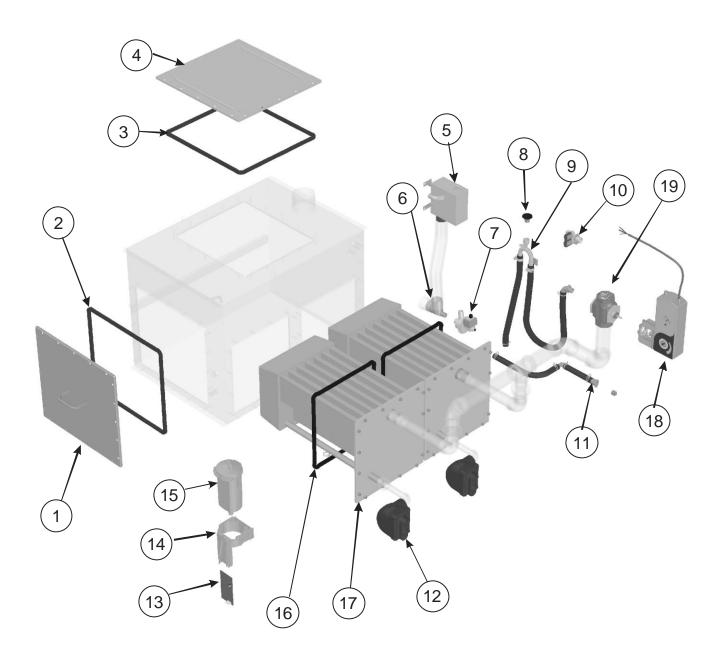
Figure 39: SETC 100-1050 Plumbing Parts
