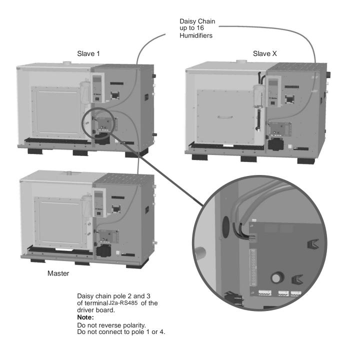
Figure 26: Staged Modulation Wiring
