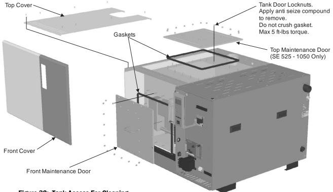
Figure 32: Tank Access For Cleaning
