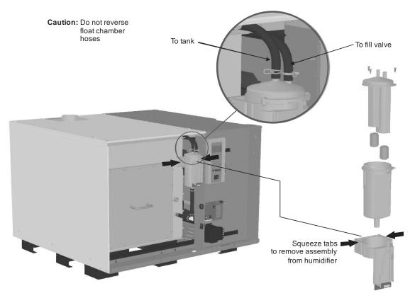
Figure 37: Float Chamber Cleaning
