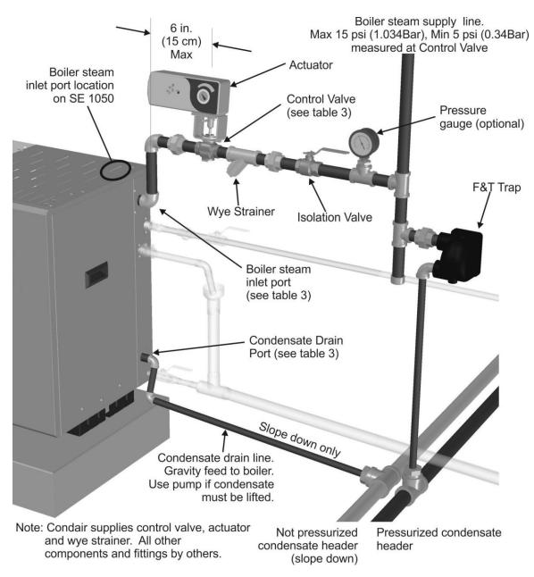
Figure 11: SE Boiler Steam and Condensate Connection
