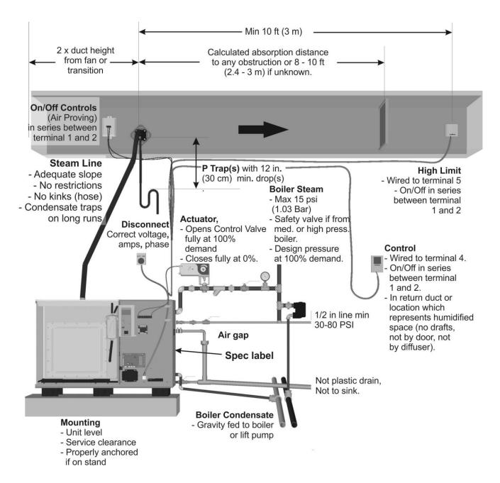
Figure 27: Installation Check
