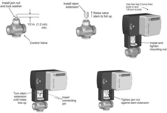
Figure 12: Control Valve Actuator Installation
