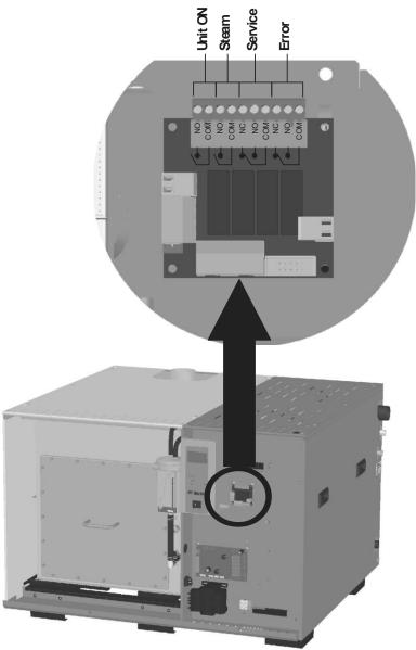
Figure 25: Remote Relay Board Wiring
