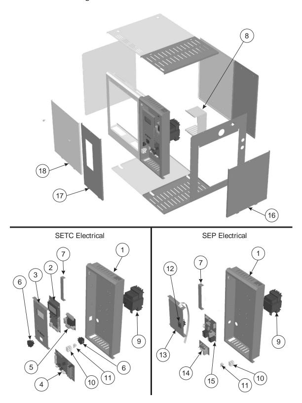
Figure 342: SETC 50 Electrical and Cabinet Parts
