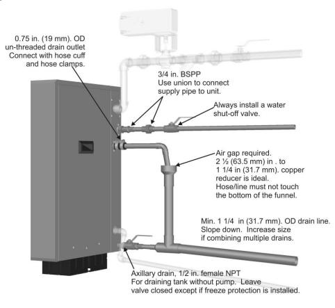
\*Pipe, unions, and water shut-off valve not supplied by CONDAIR.
