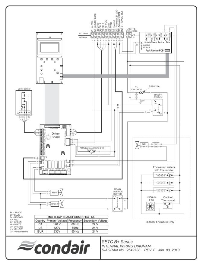
Figure 38: SETC Wiring Diagram
