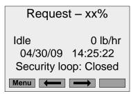
The LCD display will illuminate and the humidifier will perform a self-diagnostic sequence during which the LED's and internal components will be momentarily activated. The SE will then begin filling with water. The fill time is between 10 and 30 minutes depending on the size of the unit.
