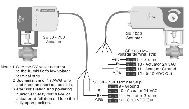
Figure 24: Control Valve Actuator Wiring
