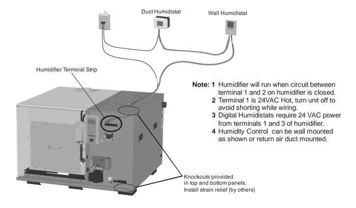
Figure 22: On/Off Controls
