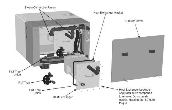
Figure 336: Heat Exchanger Removal
