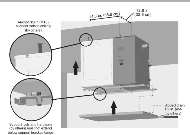
Figure 9: Ceiling Mounting the SE50
