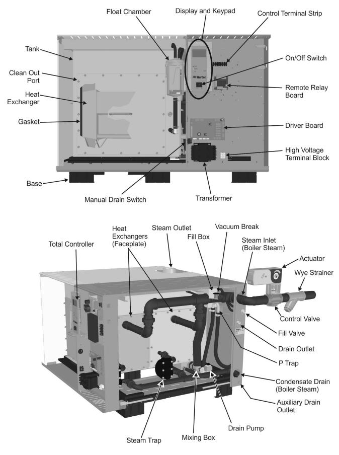
Figure 2: SETC Humidifier Components
