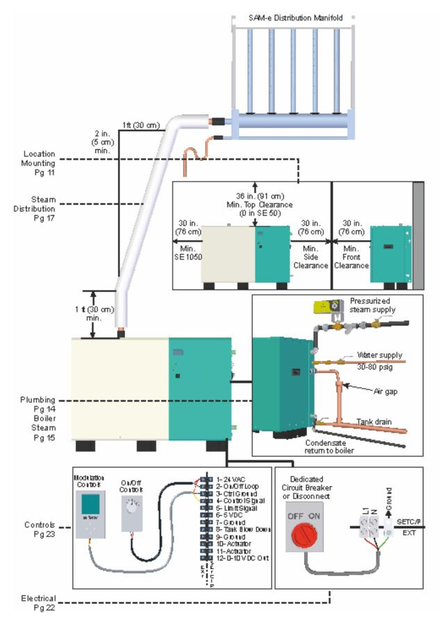
**Figure 5: Typical Humidifier Installation**
